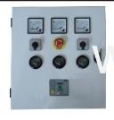
The Model 702 is a Manual Engine Control Module designed to control the engine via a key switch and pushbuttons on the front panel. The module is used to start and stop the engine and indicate fault conditions, automatically shutting down the engine and indicating the engine failure by LED, giving true, first up fault annunciation.
